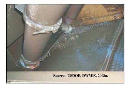
Figure 37. Shale shaker.
